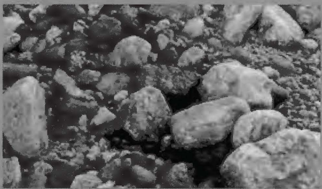
2.4 Incoherent materials include gravel and sand
