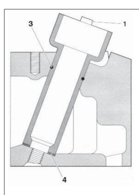
Fit a new sealing ring (4) and new copper washer (3) on the sleeve. Shear the sealing ring with low-temperature grease 1161417-9. Make sure the copper washer it securely fitted in the groove. Press down the sleeve and fit the hex socket screars and lighter them in stages to a torque of 17±1 Nm.
