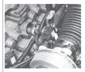
Drain the coolant from the engine and remove the spark plug as per earlier instructions.
