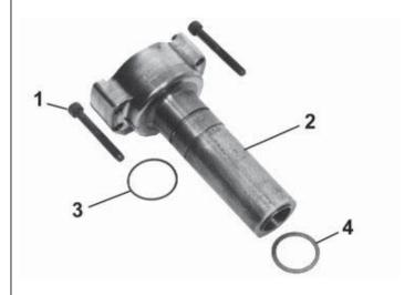
Remove the hex socket screws (1). Lever loose the spark plug sleeve (2) using two levers. Remove the sleeve, Make sure the copper washer (3) is not left in the cylinder head.
