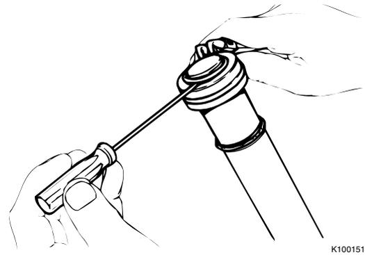
8. Tap the stop ring slightly back and remove the circlip underneath. Remove the stop ring and the top bearing from the piston rod.
