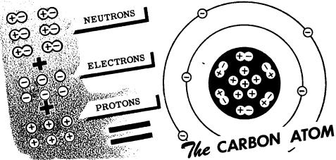
Electrons in the outer orbits of an atom are attracted to the nucleus by less force than electrons whose orbits are near the nucleus. These outer electrons are called "free" electrons and may be easily forced from their orbits, while electrons in the inner orbits are called "bound" electrons since they cannot be forced out of their orbits easily. It is the motion of the free electrons that makes up an electric current.
