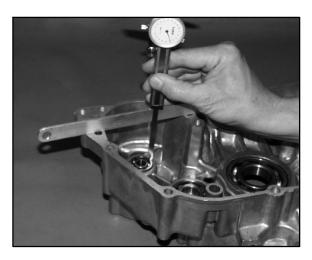
Measure the distance from the magneto crankcase mating surface to the bearing using a dial caliper and a straight edge. Subtract the thickness of the straightedge and record.
