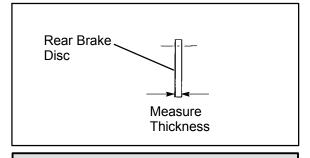
**Brake Disc Thickness**
