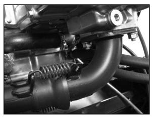
21. Remove the oil lines and breather line from the engine crankcase.
