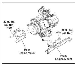
25. Carefully remove engine through top of seat base frame. Lift the engine forward to free it from the rear mount and then lift the engine out from the vehicle.
