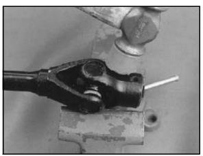
7. When installation is complete, yokes must pivot freely in all directions without binding. If the joint is stiff or binding, tap the yoke lightly to center the joint until it pivots freely in all directions.
