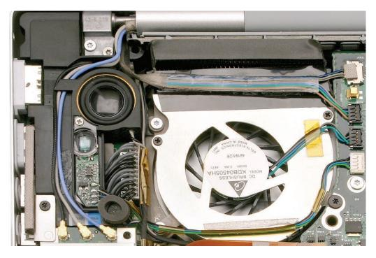
6. Connect each antenna cable to its respective terminal. Note that the color of each antenna cable corresponds with a matching color key located above the terminals.
