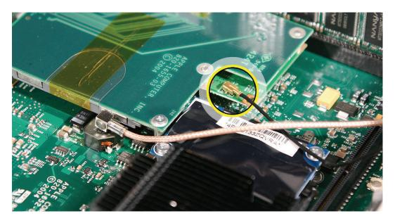
13. Remove the two screws on the mezzanine board. Lift the mezzanine board straight up and off the logic board connector. Caution: The AirPort antenna cable is still attached to the mezzanine board. Remove the AirPort antenna cable if required to perform the repair.
