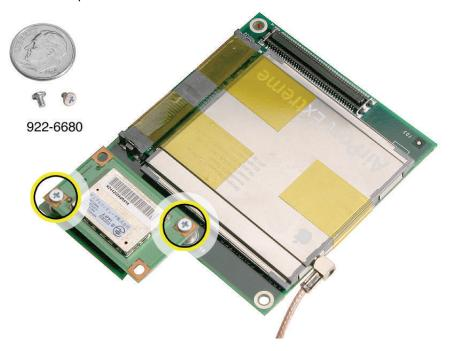
2. Connect the mezzanine board to the logic board. With a jeweler's #0 Phillips screwdriver replace the two mezzanine board screws.
