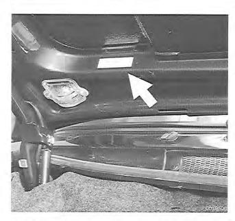
As of 1987 model year, the National Highway Traffic Safety Administration (NHTSA) requires passenger cars with a high theft rate to have the VIN marked on specific parts of the car when manufactured. On Porsche cars, these parts are identified by an adhesive label bearing the VIN and Porsche script. Replacement parts have a similar label, bearing the letters DOT-R. These labels should not be removed as they will tear apart or painted over.
