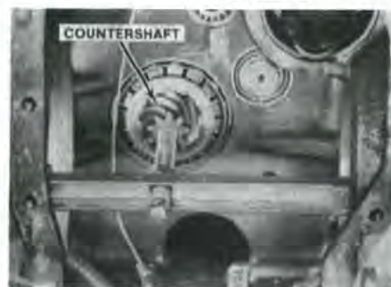
Fig. 111—With differential removed, install jackbolt and bar to support countershaft for reassembly.
