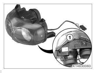
Manually adjust the headlight throw by turning adjusting screw (1).
