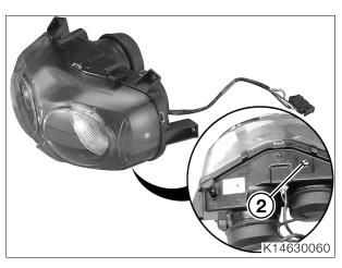
Adjust lateral throw by turning screws (2), if necessary.
