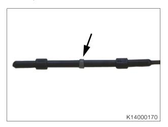
3. Top up the engine oil if necessary, but no higher than the midway mark (arrow) and repeat steps 1) to 3).
