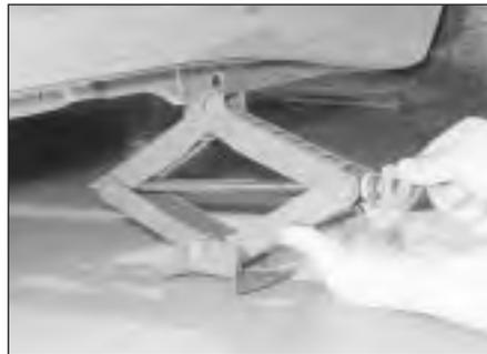
**5** Locate the jack head in the jacking point and use the brace to raise the car until the wheel is clear of the ground.
