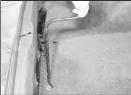
**1** In the boot, use the wheel brace to loosen the spare wheel cradle bolt.
