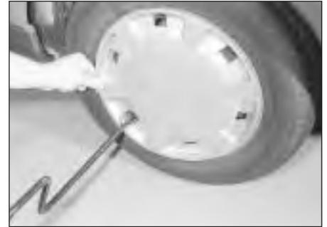
**3** Use the wheel brace to remove the wheel trim.
