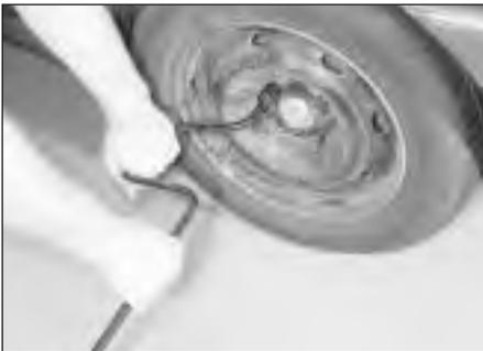
**4** Before raising the car, loosen the wheel bolts slightly using the wheelbrace.
