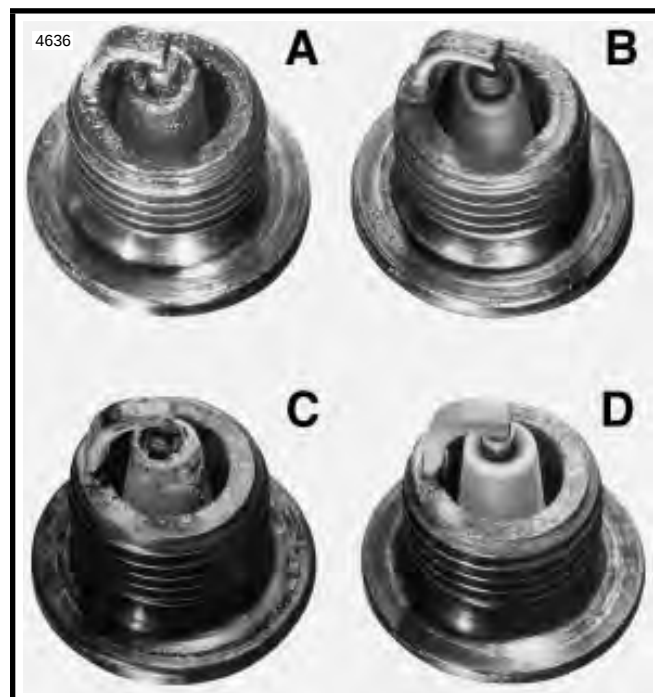
Figure 1-37. Typical Spark Plug Deposits
