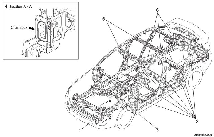
The front and rear structures to absorb high energy, and the strong and sturdy cabin structure is adopted to reduce the risk of passenger injuries at front-, rear-, and side-impact collisions, secure the space for life protection, and facilitate rescuing passengers. The structures also have the following features:
