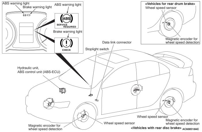
The ABS that ensures directional stability and controllability during hard braking. ABS is standard equippment on the ES and GTS models but is optional.
