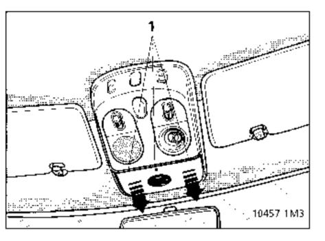
Disconnect connector (B) and remove the cap.
