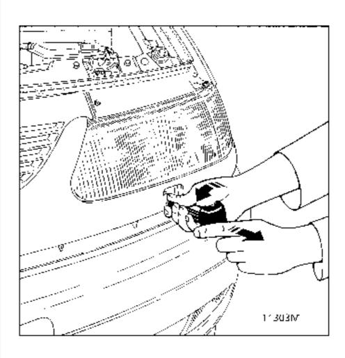
Unclip the radiator grille at both ends and remove it.
