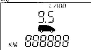
It is not displayed until the vehicle speed exceeds 25 km/h.
