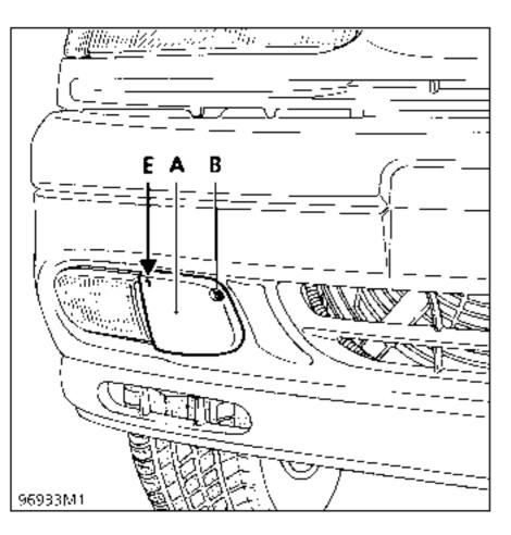
Remove cover (A) by means of bolt (B).
