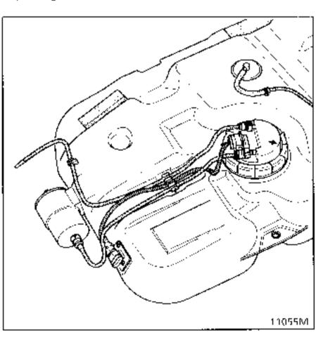
Tighten the mounting nut on the pump and sender unit assembly to a torque of **3.5 daN.m** using the tool **Mot. 1397**, holding the sender unit to prevent it from rotating.
