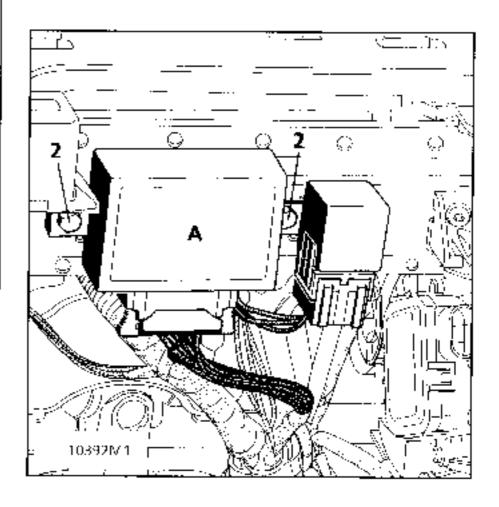
When retting, ensure that the 15-track connector is correctly clipped.
