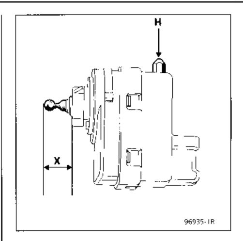
Then replace the entire receiver assembly on the lens, turning it an eighth of a turn.
