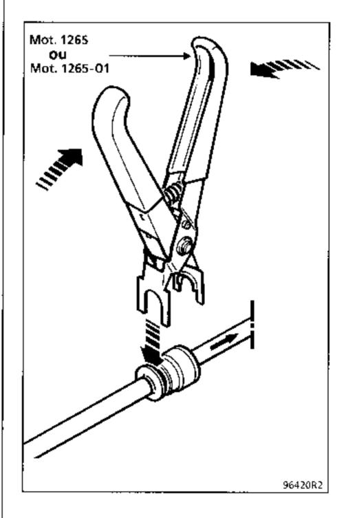
Disconnect the connector and the pipes on the sender unit side.
