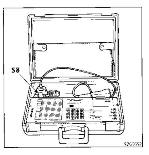
Connect the XR25 to the diagnostic socket (1) located behind the passenger compartment fuse cover under the passenger foot rest.
