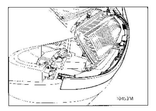
Remove the lens by its two remaining mountings (E), and if fitted with the headlight washer, remove the two mountings (F).
