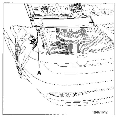
**NOTE**: To refit, proceed in the reverse order making use, if necessary, of a hook to return spring (A) to its initial position.
