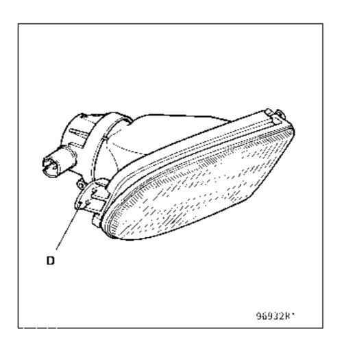
Replace the fog light by means of lug (D).
