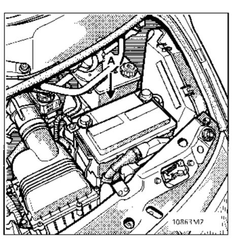
Disconnect the battery Remove the battery mounting (A)
