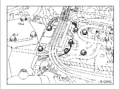
Disconnect the sensor connector (A).
